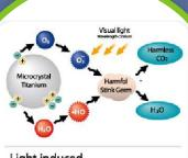
Light induced The nanoscaled particle of TiO2 absorbs visual light and becomes photocatalytic active, thus creates radicals inactivating the microbe.
